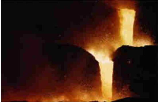
Molten metal being prepared for casting
